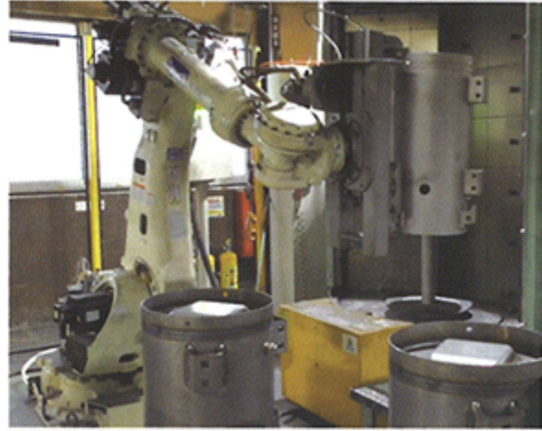
Handling for transformer case
