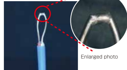
Diameter of thermocouple: 0.3 mm Welding condition: Welding current set to 2A
