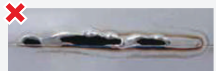
Burn-through caused by excessive heat input.
